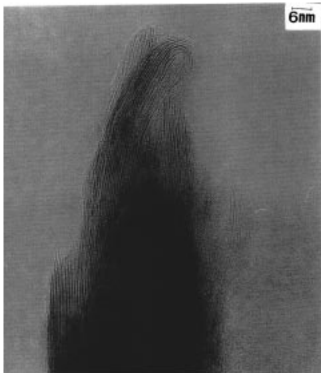
Figure 1. Transmission electron microscopy micrograph of the intercalation product of dipentylamine into molybdenum disulfide, \text{Li}_{0.1}\text{MoS}_2\{\text{C}_5\text{H}_{11}\}_2\text{NH}\}_{0.11} . The dark lines are the layers separated by about 10 Å in agreement with the d spacing observed by XRD.
